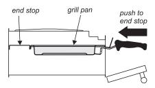
The grill pan grid can be turned over to give two grilling positions.
